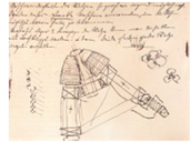
Cross-rolling process sketch of Max Mannesmann, pre 1885
